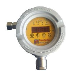
Detector has provision to set Two alarm levels of warnings (High & Low).
