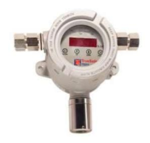
Relay output is provided and this output can be connected to the conventional Gas Detection Panel OR SCADA system. For BMS connectivity detector has provided RS485 output. Additionally 4-20mA and Selectable 0-5 V & 0-10V Analog output could be also available. Enclosure used is suitable for Zone 1 & Zone 2 hazardous areas.
